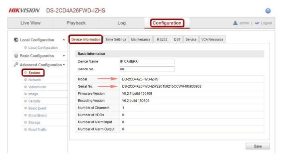
2. Camera firmware/encoding number and build.
