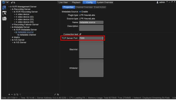
**d.** Users can add corresponding metadata channels and define "Camera ID" for receiving the detection results from multiple channels. (The ID of a camera is defined by Neural Labs VPAR system and can be found in Camera Management > Select Camera > ID)
