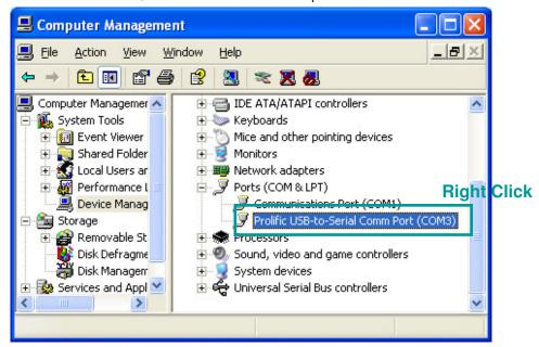
2. Choose Properties > Port Setting. The value of "Bit per second" is the value of this device's Baud rate.
