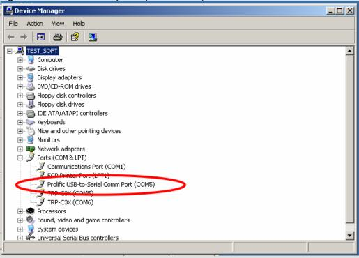
4. If the device was completely installed you can see new COM devices listed. This means Windows has assigned the device to the COM# port.
