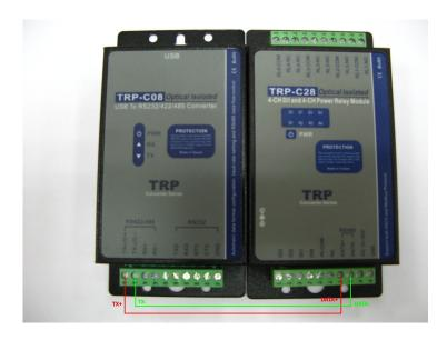
Step 2: Install the driver of SCB-C08 in the desktop. Connect between SCB-C08 and the desktop. (Please refer to "C08\_manual\_Eng.pdf" in the folder "C08" for more installation details.)
