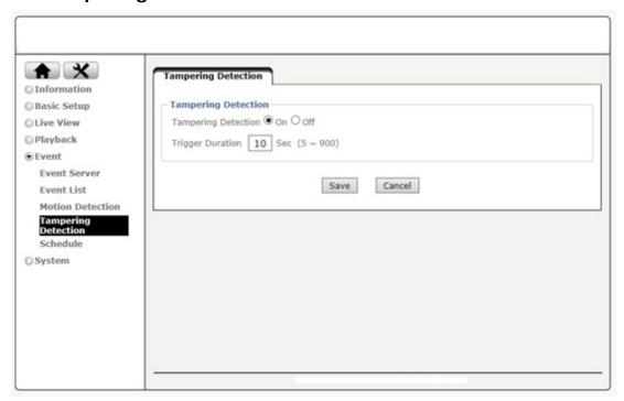
If the image of the camera is obstructed, e.g., because someone covers up the lens or moves the image out of focus, the camera notices this and generates a trigger alert. You can define how long you want the alert state to remain active after the event has occurred.
