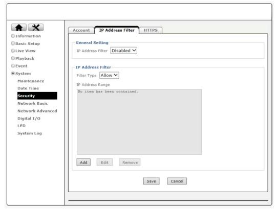
Once you enabled it, the listed IP address are allowed or denied access to the network camera. Add the IP address that you'd like to allow or deny, select allow or deny from the list and save it.
