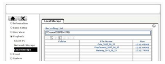
If your camera is equipped with a local storage option (recording on an SC card) you can access the recordings from here. It functions similarly to the access of files on the network storage device.
