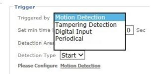
movements and triggers an alert when it detects motion. Motion detection needs to be configured first for that to work.
