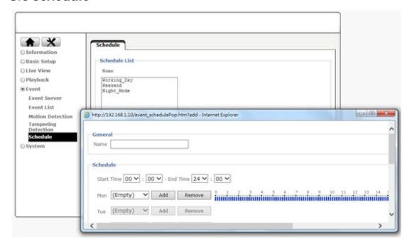
The Network Camera supports event trigger actions that can be based on a schedule. This can be used, as an example, to only activate motion detection between 9 pm and 6 am during business days and around the clock on the weekends. You can set up individual schedules for
