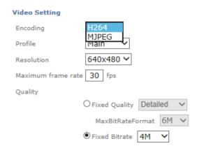
**Profile-** Encoding applications offer you the choice between Main and High profiles. High is more complex than Main, and produces a broadcast quality output.
