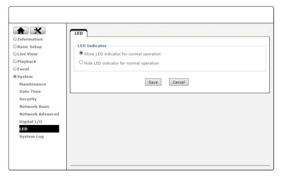
You can enable or disable the operation LEDs on your network camera. Hiding the LED indicator will make the camera appear to be offline while in fact it is operational and captures video.
