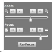
**Re-Focus-** The faster way to find the best focus. We suggest you click Re-Focus button to automatically find the appropriate focus value and click arrowhead of zoom or focus to do slight adjustment.
