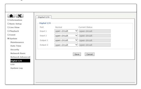
If your network camera is equipped with a digital I/O interface, you can configure the connections on this page. The screen shows the current status of input 1 and output 1. The screen also allows you to define the "normal" state of the port. The normal state can be viewed as the "non-alert-state."
