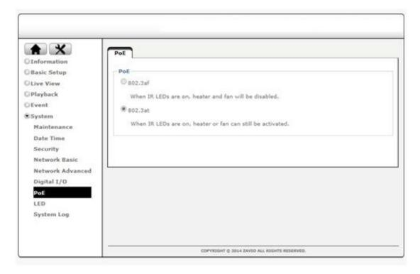
When you empower IP Camera, the system will detect af/ at mode of PoE automatically.
