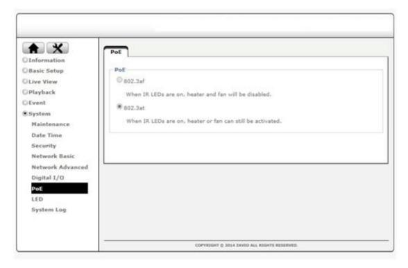
When you empower IP Camera, the system will detect af/ at mode of PoE automatically.
