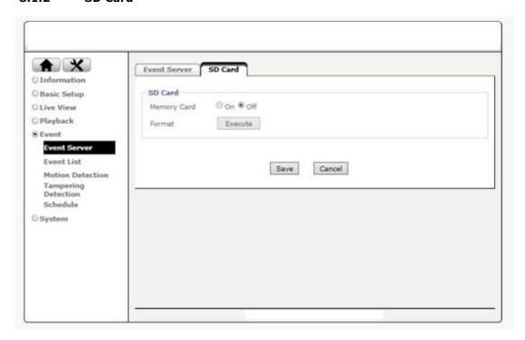
If you want to record video footage on a local SD card, you first must insert the SD card (see hardware installation guide for details), and then you must set the Memory Card to "on" and format the card by clicking "Execute."
