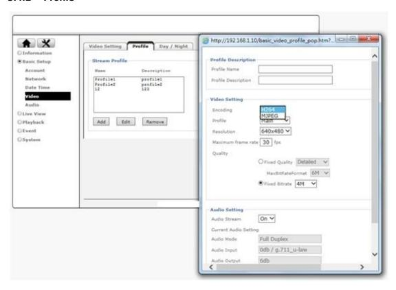
The network camera allows the creation of video streaming profiles. For each profile you can define the video resolution, the viewing area and the video codec that is to be used. Click "Add" to create a new profile, "Remove" to delete a profile or "Edit" to modify an existing profile.
