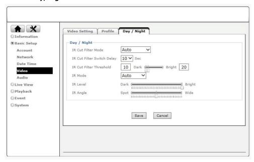
Some network cameras are equipped with active IR LEDs providing the ability to capture video in complete darkness. Note, that if your camera is not equipped with IR LEDs, this menu will not be available. Also note that some menu items will vary depending on your camera model.
