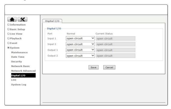
If your network camera is equipped with a digital I/O interface, you can configure the connections on this page. The screen shows the current status of input 1/ input 2 and output 1/ output 2. The screen also allows you to define the "normal" state of the port. The normal state can be viewed as the "non-alert-state."
