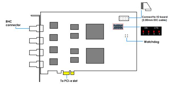
**Note:** The default configuration of the black switch on 8004HD card is as above. Do not adjust it.
