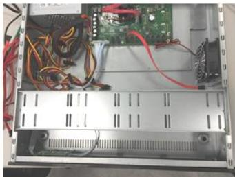
1. Dismantle the HDD bracket from the cabinet.
