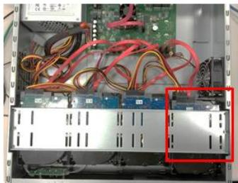
3. Assemble the HDD bracket back to the cabinet and insert the SATA cables and power cable.
