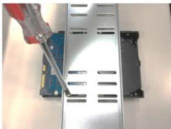
2. Put HDD under the bracket and install HDD on the bracket with 4 screws.
